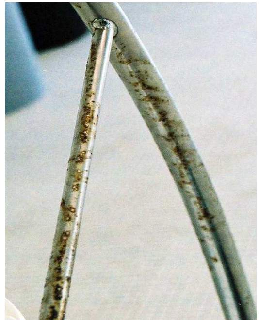
Figure 4: This chrome plated carbon steel reel for holding lane markers has only been in use for a few years but there has already been substantial corrosion under the plating. Photo Courtesy of TMR Consulting.
